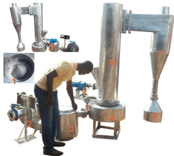
1– The interior view of the dryer basement, 2– the blower, 3– the heating chamber, T– temperature indicator, 4– the dryer basement, 5– the feeder, 6– dryer column, 7– the cyclone, 8– product collector
