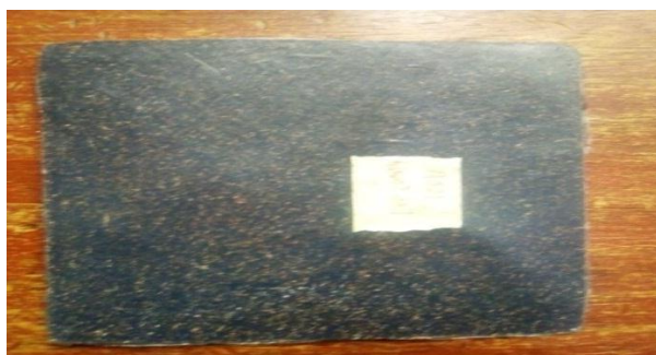
Plate 3.2: 75wt% rLDPE reinforced with 25wt% Raw Untreated EGS
