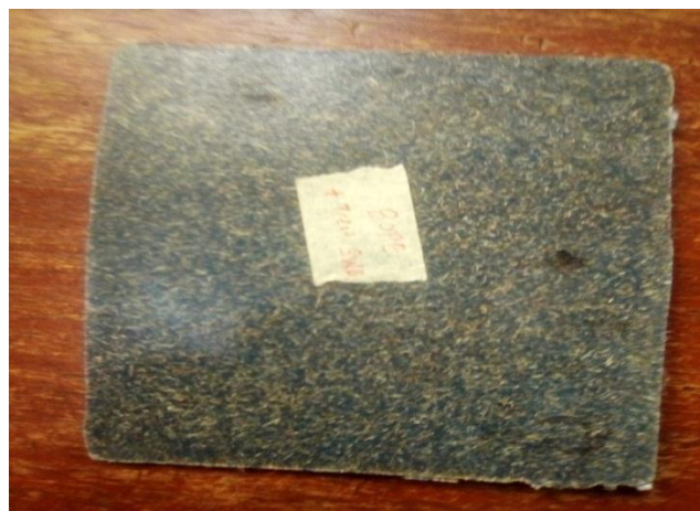
Plate 3.3: 85% rLDPE Reinforced with 15% Treated EGS
