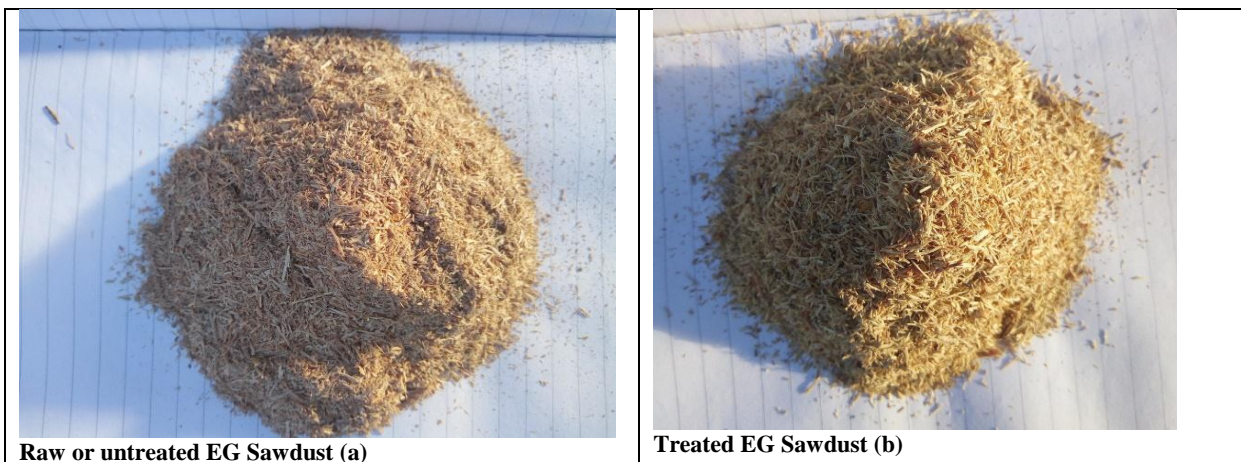
Plate 2.1: Raw untreated (a) and Treated (b) EG Sawdust
