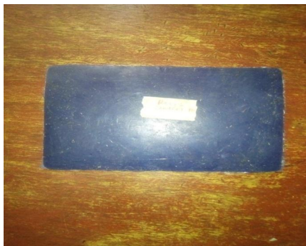
Plate 3.1: 100wt% Recycled Polyethylene Matrix (Control)
