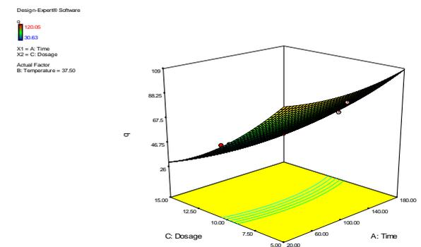
**Figure 8:** Response Surface Combined Effect Plot of Dosage (g) and Time (min) Variables for Uptake of Zinc Ions by Sorbent.
