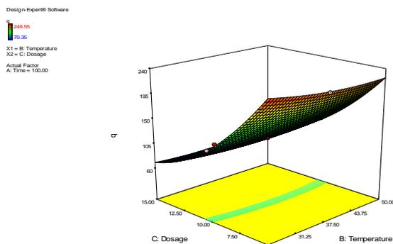
**Figure 5:** Response Surface Combined Effect Plot of Dosage (g) and Temperature (°C) Variables for Uptake of Iron Ions by Sorbent.
