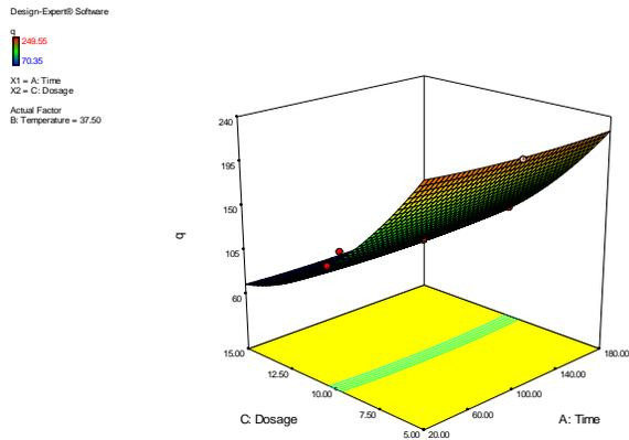
**Figure 4:** Response Surface Combined Effect Plot of Dosage (g) and Time (min) Variables for Uptake of Iron Ions by Sorbent.
