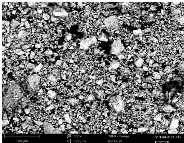
**Plate 1:** SEM Image of Immobilized Baker's Yeast before Sorption at 500 x magnification
