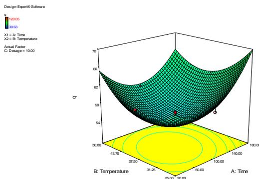
**Figure 10:** Response Surface Combined Effect Plot of Temperature ( $^{\circ}\text{C}$ ) and Time (min) Variables for Uptake of Zinc Ions by Sorbent.
