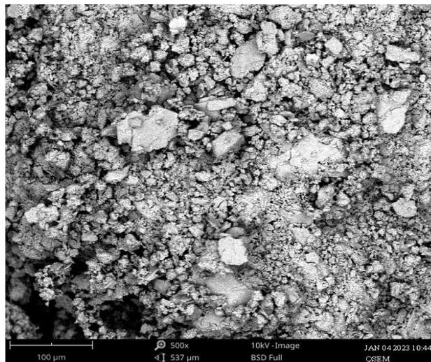
**Plate 2:** SEM Image of Immobilized Baker's Yeast after Sorption at 500 x magnification
