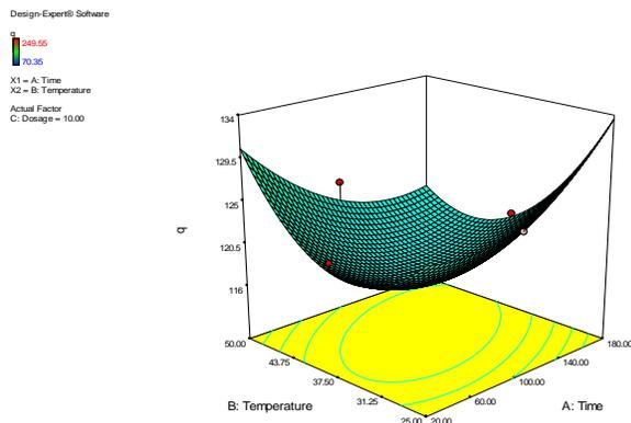
**Figure 6:** Response Surface Combined Effect Plot of Temperature (°C) and Time (min) Variables for Uptake of Iron Ions by Sorbent.
