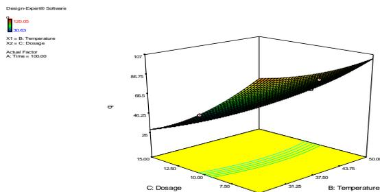
**Figure 9:** Response Surface Combined Effect Plot of Dosage (g) and Temperature ( $^{\circ}\text{C}$ ) Variables for Uptake of Zinc Ions by Sorbent.
